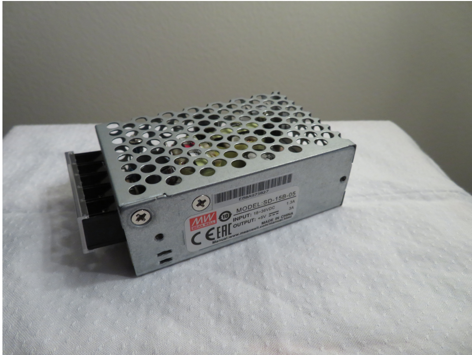
Figure 3.10: The Meanwell SD-15B-05 is able to provide 5V at up to 15W, well suited for the demands of the APMS.
