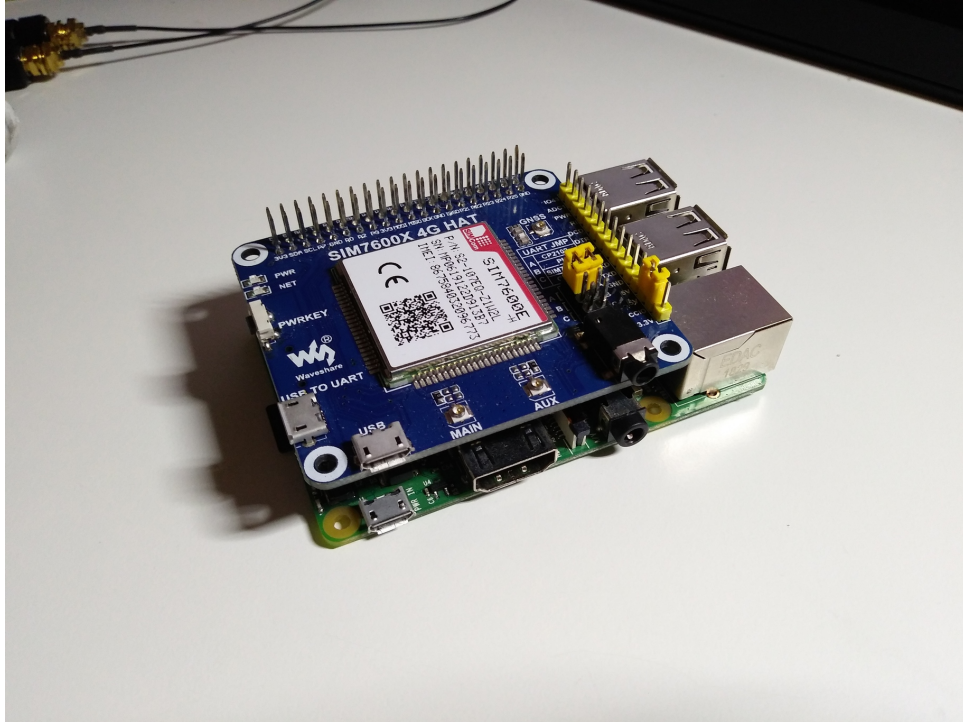
Figure A.1: Connect the SIM7600E to the Raspberry Pi, ensuring the entire row of headers is attached firmly
