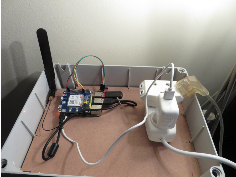
Figure 5.1: APMS as modified for testing. Note the use of a conventional AC-DC powersupply
