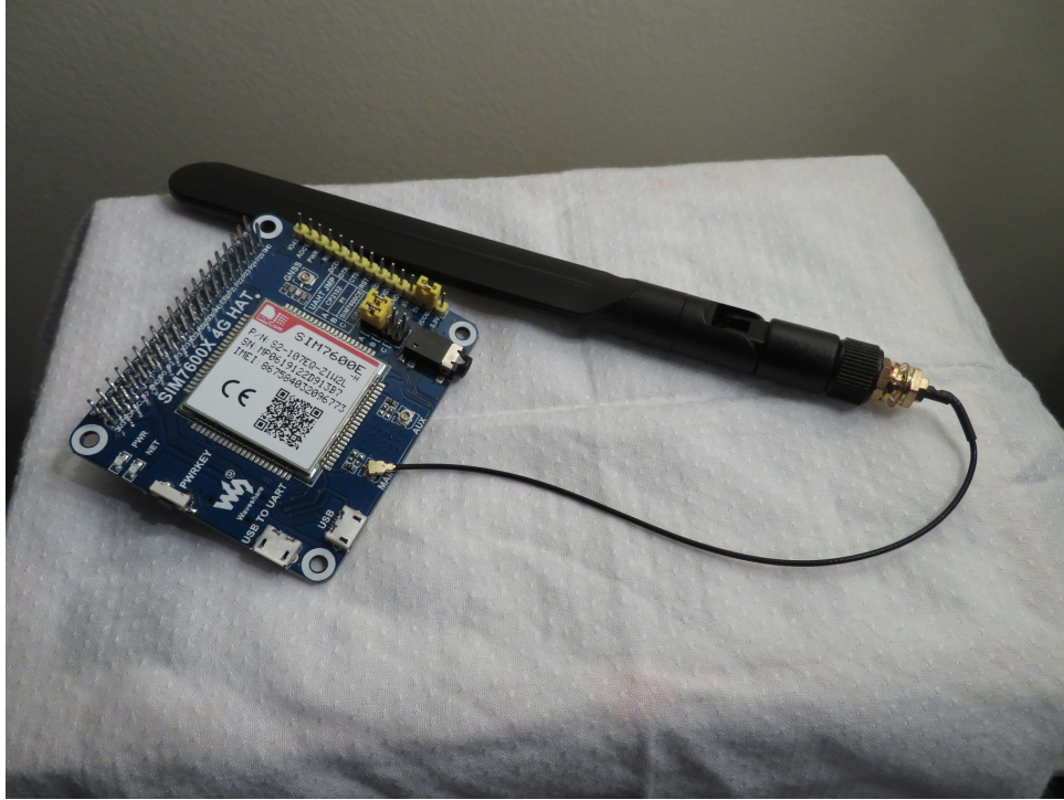
Figure 3.4: The SIM7600E is a 4G capable cellular modem with the ability to present as a QMI network device to a variety of systems.
